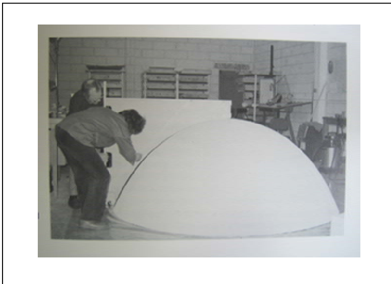
Figure 1. The work on the dome made of Styrofoam.
