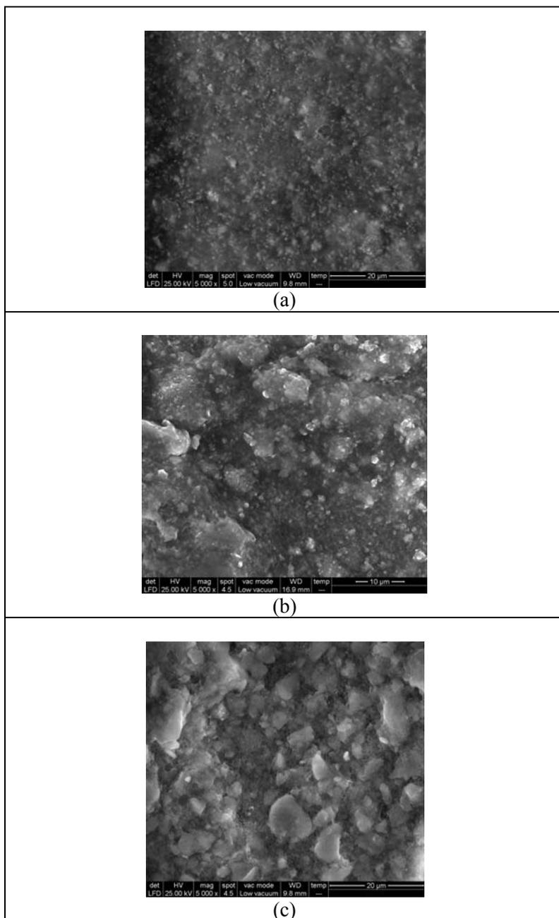
**Figure 2.** SEM images of studied pigments after 1 h of treatment in HF plasma: (a) yellow pigment, (b) red pigment and (c) green pigment.
