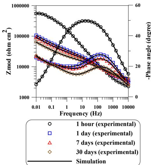
**Figure 4.** Bode plots for electrochemically patinated bronze recorded at open circuit potential, after different time of immersion in simulated acid rain.
