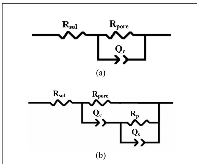
**Figure 5.** Equivalent circuits used for fitting the measured impedance spectra.
