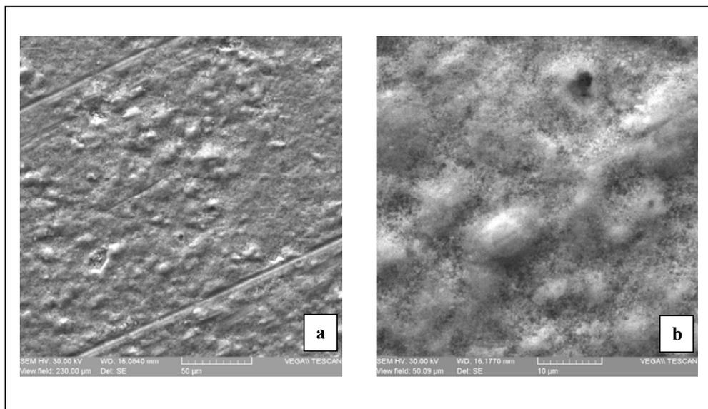
**Figure 1.** SEM micrographs of the electrochemically patina formation on bronze substrate.
