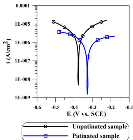
**Figure 3.** Potentiodynamic polarization curves for unpatinated and patinated bronze samples after 1 hour immersion in simulated acid rain; 1 mV/s and 20° C.
