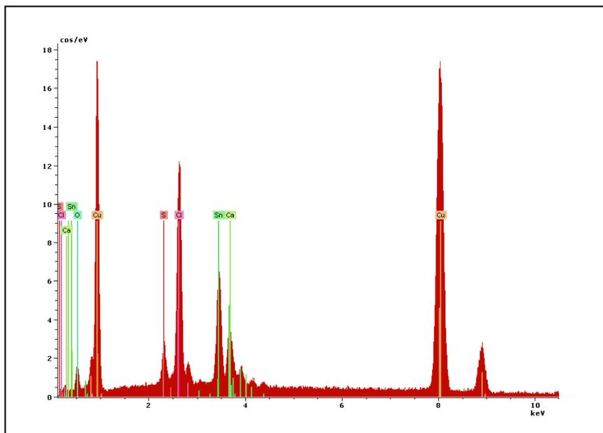
**Figure 2.** EDX spectrum for the electrochemically patinated bronze surface.
