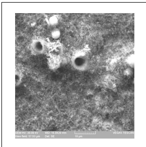
**Figure 6.** SEM observation of the patinated sample after 30 days immersion in simulated acid rain.
