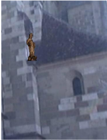
Figure 4. Co-location of the reconstructed virtual model with the ‘Black Church’ using the developed AR system.
