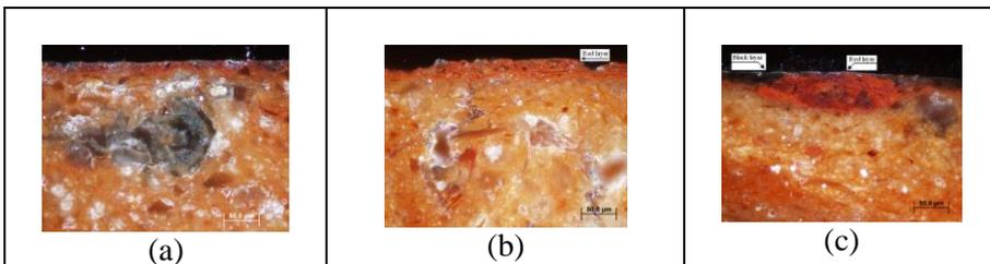
**Figure 4.** Cross section microphotographs in visible light at  $\times 500$  magnification of samples a) GA33<sup>b</sup>, b) GA42<sup>b</sup>, c) GA35<sup>b</sup>.
