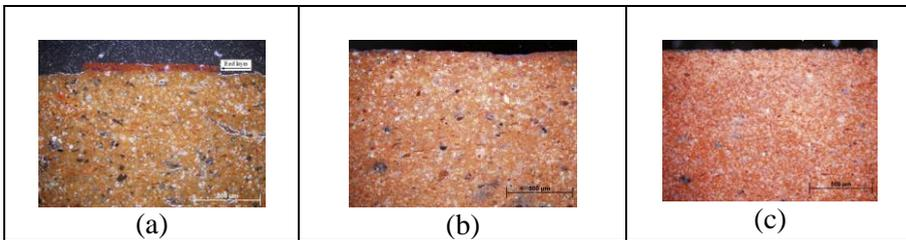
**Figure 3.** Thin and cross-section microphotographs in visible light at  $\times 100$  magnification of samples a) GA13<sup>a</sup>, b) GA33<sup>b</sup>, c) GF66<sup>a</sup>.
