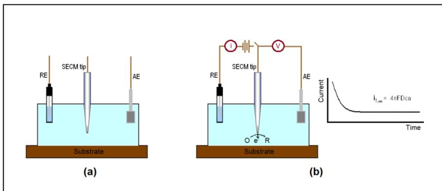
**Figure 2.** Sketch of an electrochemical scanning microscope: (a) the UME is immersed in a solution containing a redox species  $O$ , (b) the potential at the UME is set to a value at which the species  $O$  can be reduced to  $R$  under diffusion limiting conditions. The current trace recorded at the UME in the later condition is also given.
