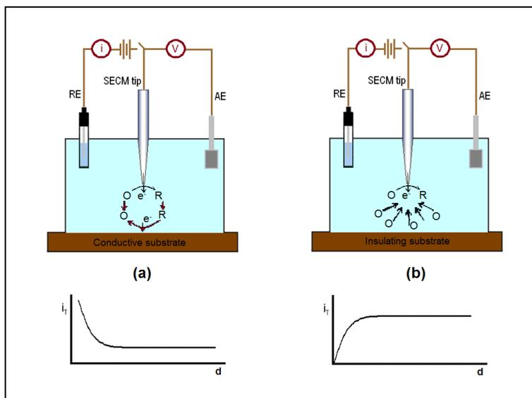
**Figure 3.** Basic principle of SECM: (a) positive feedback - the tip is located near a conductive substrate where the oxidation of species  $R$  occurs; (b) negative feedback: the tip is placed near an insulating substrate which hinders the diffusion of species  $O$ .
