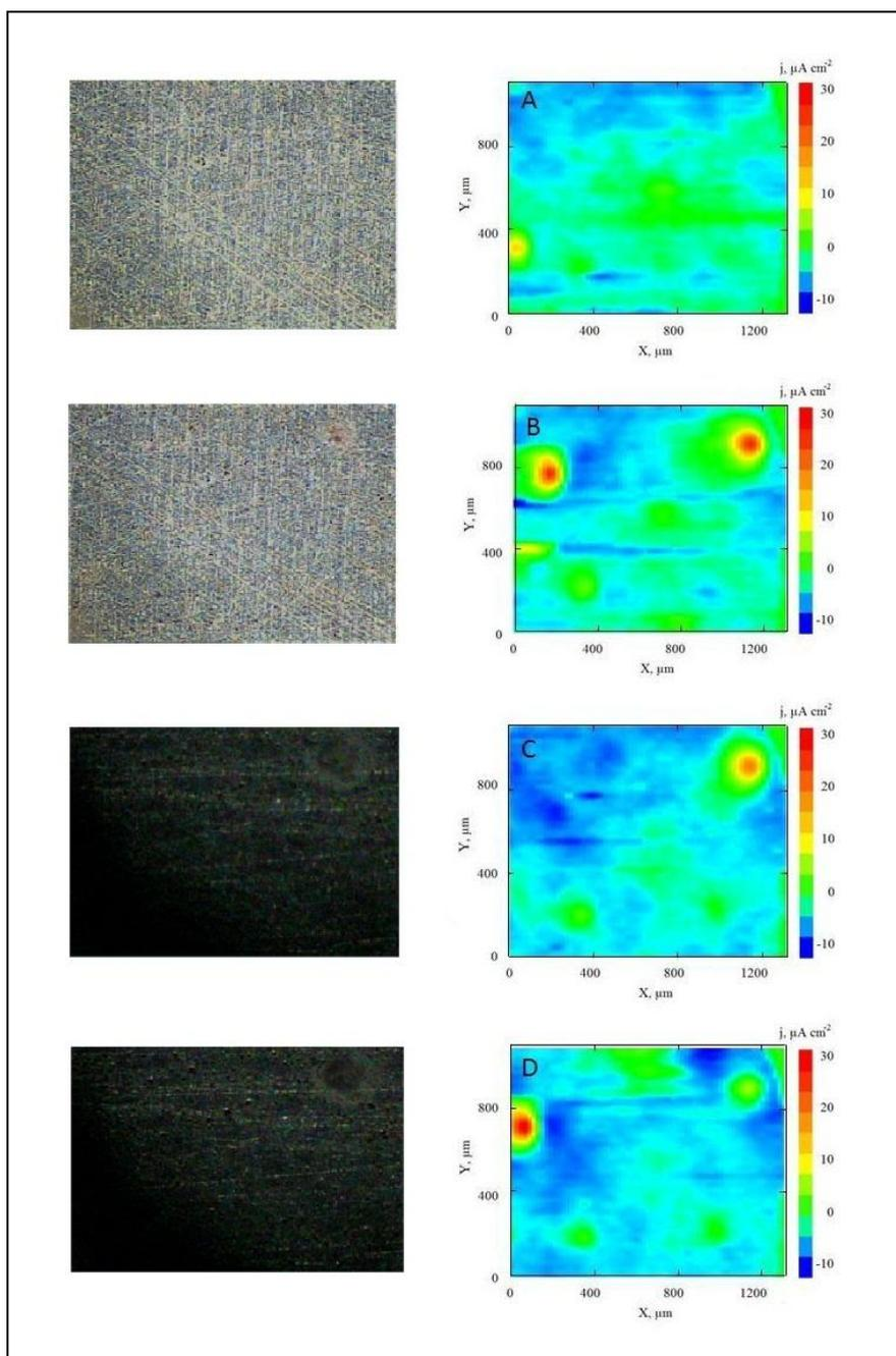
**Figure 10.** SVET images and micrographs of AA2024 alloy immersed in 50 mM NaCl aqueous solution for: (a) 4, (b) 5, (c) 9, and (D) 11 hours. Values of Z axis: Ionic current,  $\mu\text{A cm}^{-2}$ . Tip-substrate distance: 50  $\mu\text{m}$ . The images represent 1000  $\mu\text{m}$  x 1300  $\mu\text{m}$  in X and Y directions.
