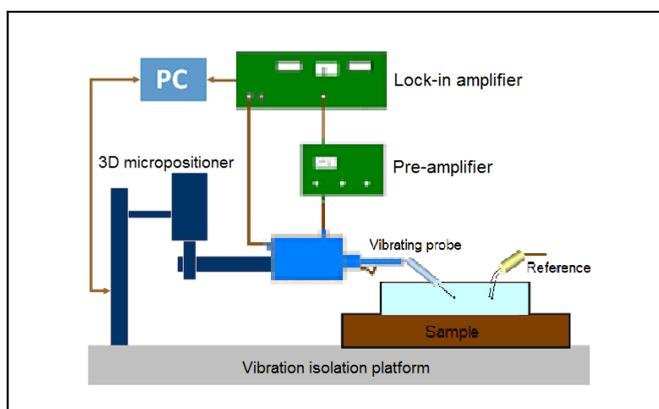
**Figure 9.** Scheme of the basic components of a SVET equipment, including the components of the electrochemical cell and their general function.
