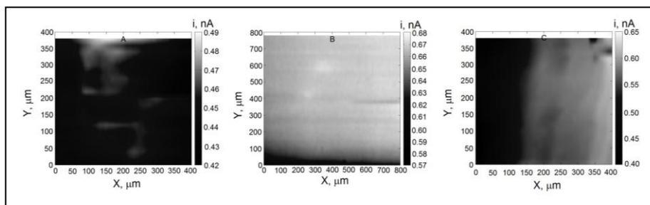
**Figure 5.** SECM images of steel substrates painted by an epoxy coating after 24 hours immersion in: (a) pure water, (b) 0.05 M NaCl, and (c) 0.5 M NaCl solutions. 0.5 mM ferrocene-methanol was added to the test solutions as redox mediator. Values of Z axis: Current, nA. Redox mediator: oxygen. Tip potential: +0.50 V vs. Ag/AgCl/KCl (saturated) reference electrode. Tip diameter: 10  $\mu\text{m}$ . Tip-substrate distance: 15  $\mu\text{m}$ .
