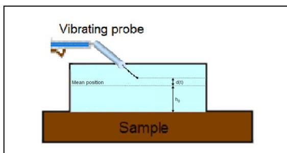
**Figure 8.** Sketch of the scanning vibrating electrode technique. The Pt microelectrode is vibrated perpendicular to the surface of the investigated substrate while immersed in a solution of low conductivity.
