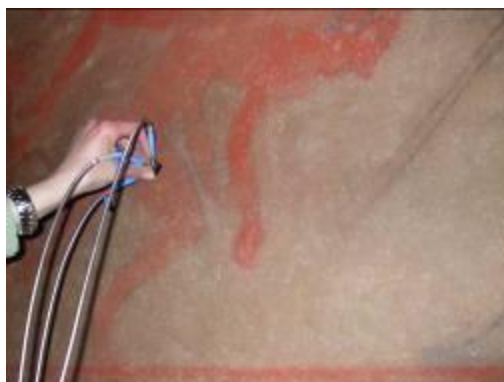
Figure 4. Color measurement of one selected area: (a) using the masks held in place by hand, and (b) a detail of the head of the colorimeter in the acquisition phase.
