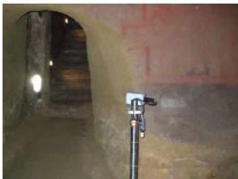
Figure 2. Climatic station for controlling temperature and relative humidity, placed in the atrium of the Tomba della Scimmia .
