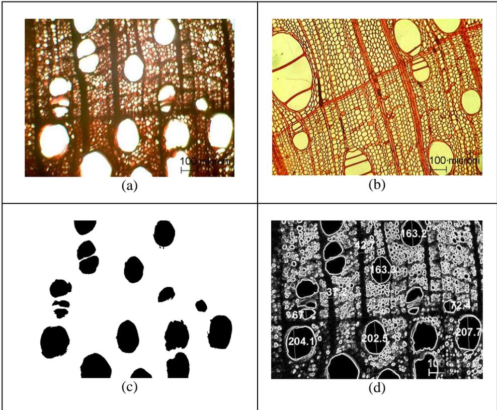
**Figure 6.** Cross sections: (a) investigated sample J3 - magnif.100x, (b) reference sample (walnut - *Juglans regia*) - 100x, (c) 'mask' image of the investigated sample J3 - 100x (size 1312.96x983.33  $\mu\text{m}$ ), (d) investigated sample - cell contour enhanced and measurements - 100x; e-investigated sample J3 – magnif. 200x (size 656.48x491.67  $\mu\text{m}$ ); f-reference sample (walnut- *Juglans regia*), 200x
