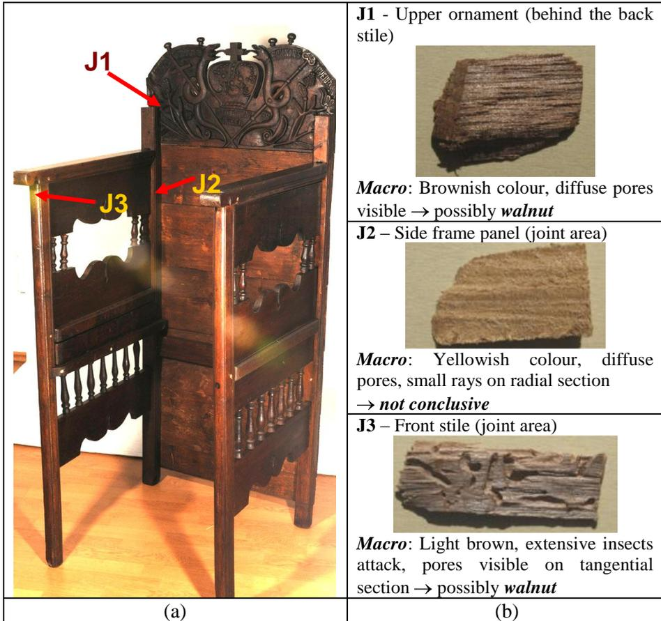
**Figure 1.** The object (a) and samples taken out for investigation (b): aspect, macroscopic features and presumptive identification; red arrows are pointing towards the elements and areas where from the samples J1, J2, J3 were taken out.
