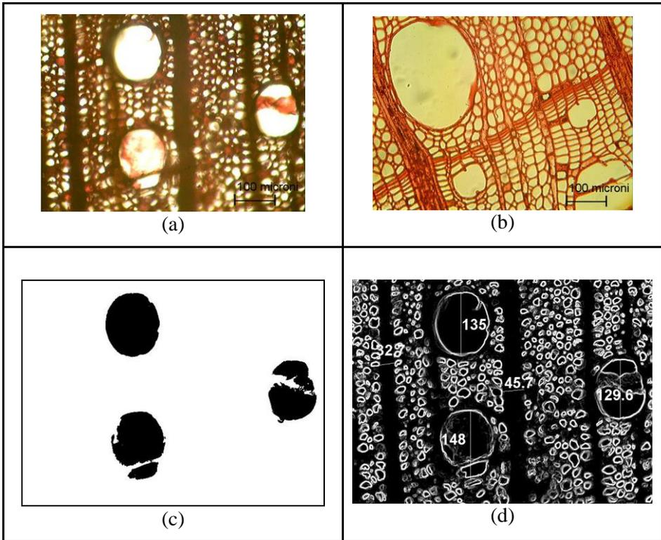
**Figure 2.** Cross sections, magnification 200x: (a) investigated sample J1, (b) reference sample (walnut - *Juglans regia*), (c) 'mask' image of the investigated sample J1, (d) investigated sample J1 with cell contour enhanced and measurements. Size of the investigated sample micrograph: 456.48x491.67 ( $\mu\text{m}$ ).
