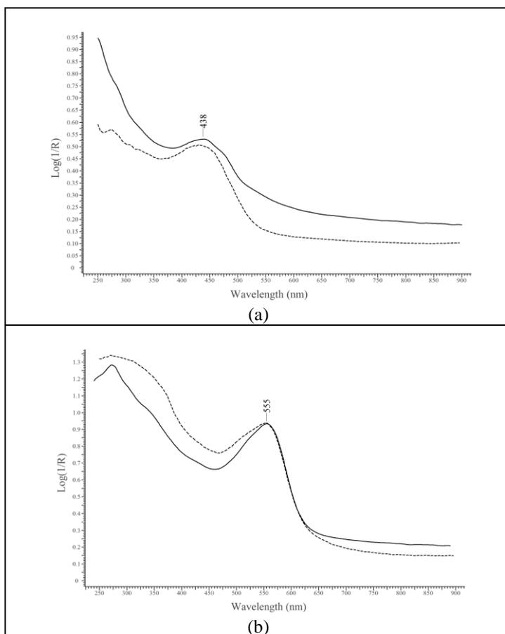
**Figure 4.** FORS spectra of non-written folios: (a) saffron (dashed line) and (b) brazilwood (dashed line) against their respective standards (solid line).
