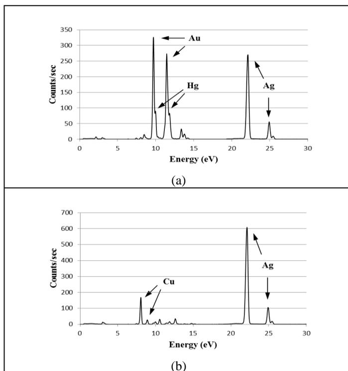
Figure 3. XRF spectra from the binding of ms. 3290: (a) background gilded silver and (b) black *niello* decorations.
