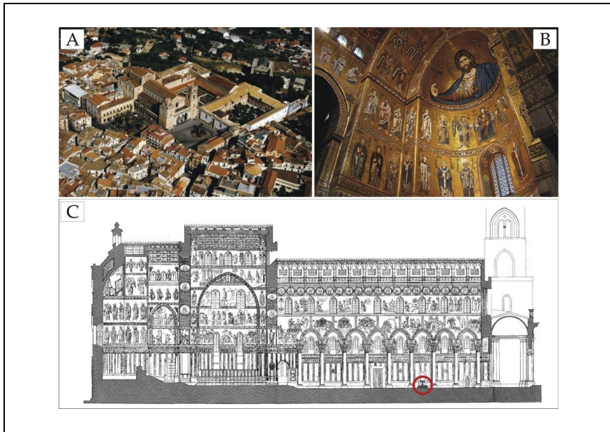
Figure 1. (A) Aerial view of the Monreale Cathedral, (B) central apse with mosaic decorations, (C) cross section with the present position of the Baptismal Font (red circle).
