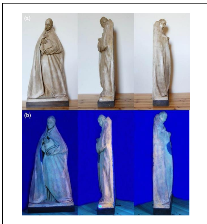
Figure 3. Photographs of the model of Saint Alphonsus: (a) visible and (b) UVF.
