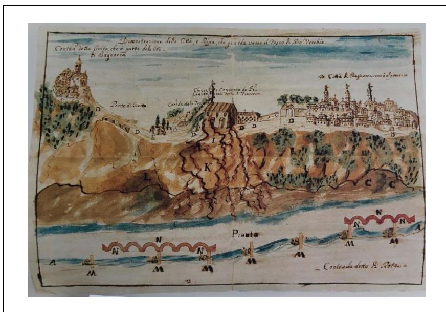
Figure 4. Drawing representing a view of the Bagnoregio and Civita area with particular reference to geomorphological instability and planned hydraulic measures. This drawing, by F. Antonini, was enclosed to the relation sent by Bagnoregio Municipality to the Sacra Congregazione del Buon Governo of Rome in 1765 [A.C.B. Liber consiliorum , c. 19t,15/12/1765].
