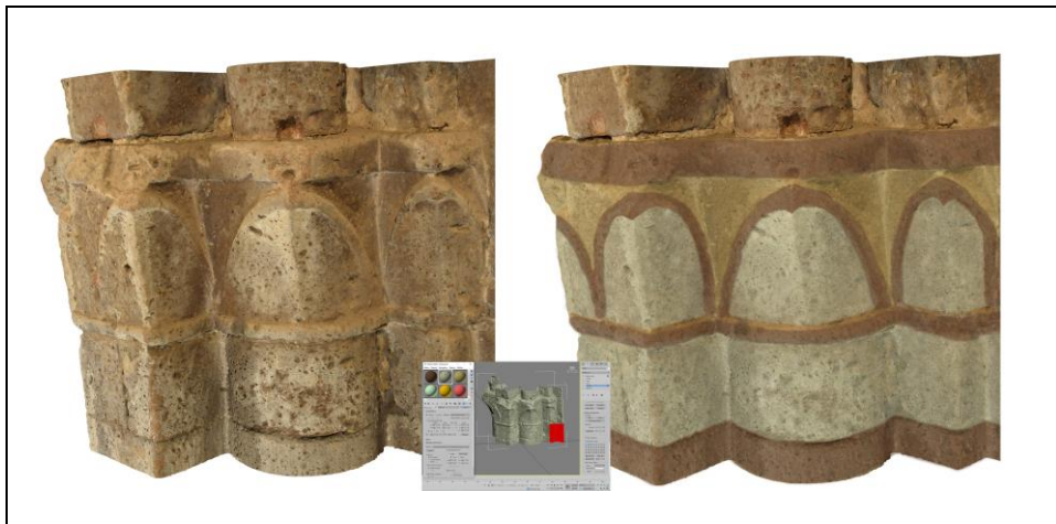
Figure 6. 3D photogrammetric model (left) and mesh texturized by detected colours (right). The GUI (Graphic User Interface) of 3DS Max is also shown in the figure.
