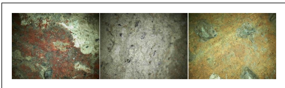
Figure 4. Videomicroscope acquisitions of red, white and yellow colours at magnification 50x.
