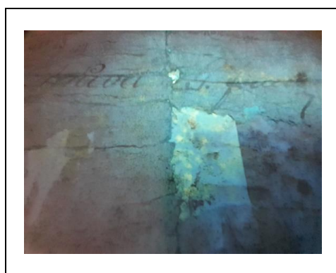
Figure 4. Greenish fluorescence observed on empirical restoration area with UV light lamp (365 nm).
